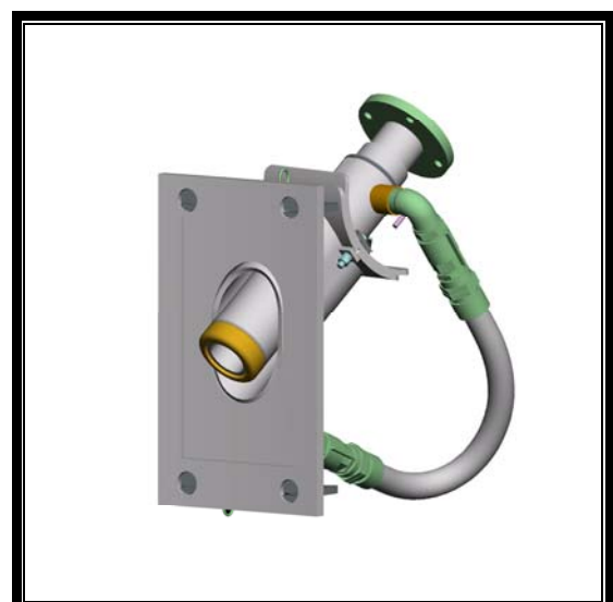
Figure 4. Sidewall injector design Courtesy: More' srl
